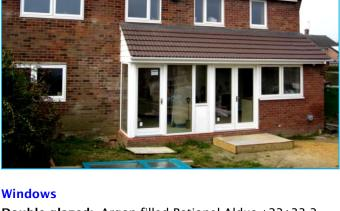
Double glazed: Argon-filled Rationel Aldus +22+33.2 thermofloat U\_=1.16Ar, aluminium clad, timber framed www.rationel.co.uk
